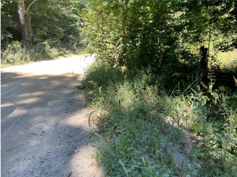
Photo 8: River Front Drive, facing west along south side of access road. Fill encroachment into adjacent wetland was noted in the field.
